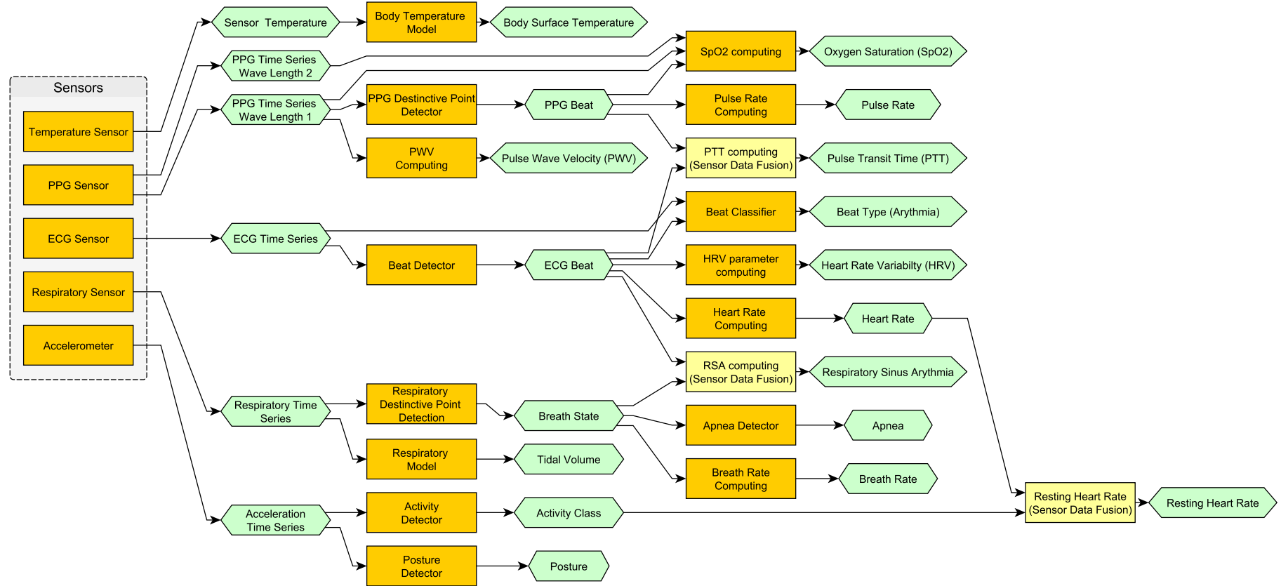
Figure 2.6.: A signal flow diagram with the sensors at the left side followed by their time series, algorithms, and computed data. Signal processing blocks are represented in squared blocks. Signals themselves are represented as hexagonal blocks. A detailed definition for this type of signal flow diagram is included in the appendix A.
