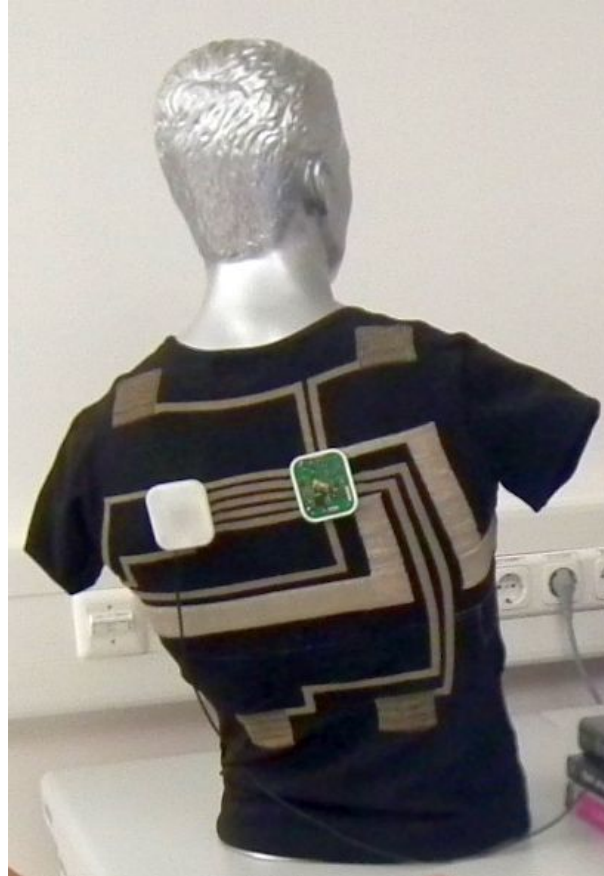
Figure 2.2.: Wearable research example: Additive manufactured wearable shirt with fabric ECG electrodes and fabric respiratory sensor developed at the Fraunhofer IIS in Erlangen [146]. This fabric was woven in one work cycle using an elastic non-conductive fabric and two different types of conductive fabrics for sensors and electric leads.
